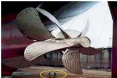
Contra Rotating Propeller (출처: Marine engineering)
